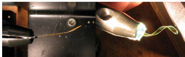
Figure 27. A nematic network photo-cantilever with a twist director distribution through its section curls (right) on illumination (18).
